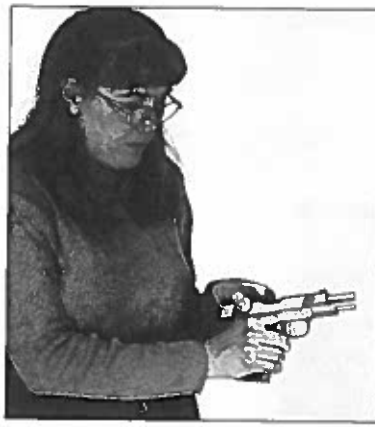
Always function check a firearm without ammunition after it has been disassembled for cleaning or repair. Here a shooter works the slide of a semi-automatic pistol.
